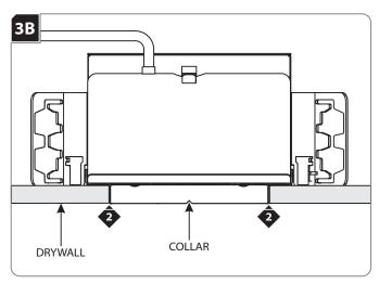
Align the cut out section of drywall with the collar and install drywall.
